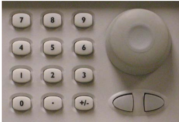
Fig. 5. Signal Generator Amplitude and Frequency Adjustment Controls
